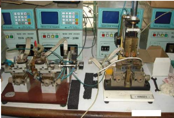
Close loop “Ti” Welding Setups.
